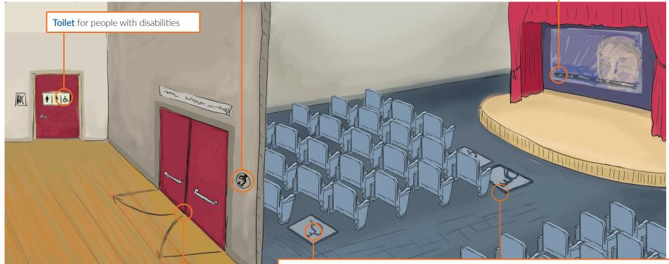
**Easy access**, door still height max 2 cm and not sharp. Marking for the opening direction of the doors
